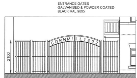
ENTRANCE GATE ELEVATION SCALE 1:50
